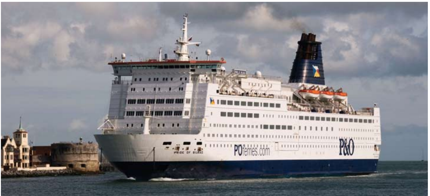
ABOVE: P&O's 37,583ft Pride of Bilbao was built in 1986 as Olympia by Oy Wärtsilä, Turku, Finland and can carry 580 cars and 77 lorries on her vehicle decks.
